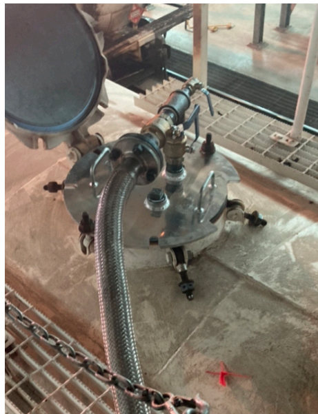
3D Rotary Orbital Sprayer – Fastened in the manway, the sprayer rotates a full 360 degrees and sprays down the tank car in 20 minutes
