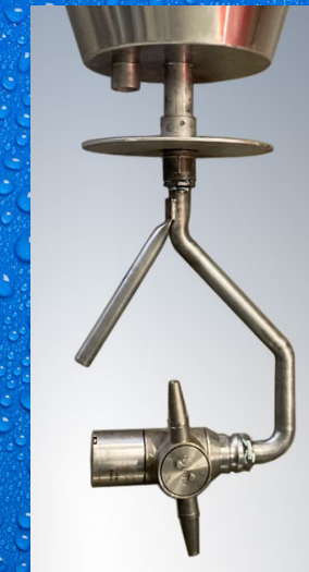
3D Rotary Orbital Sprayer – Fastened in the manway, the sprayer rotates a full 360 degrees and sprays down the tank car in 20 minutes
